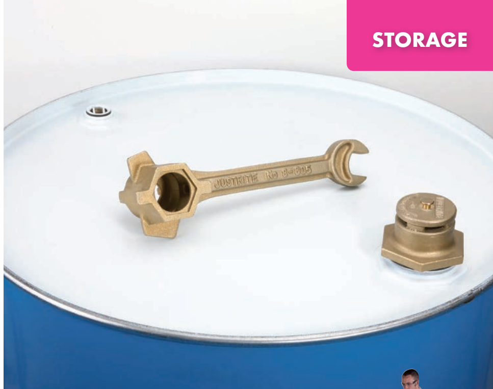
Above: Vent on a vertically stored drum provides automatic relief of both pressure and vacuum. A nonsparking drum wrench safely opens tight bungs.
