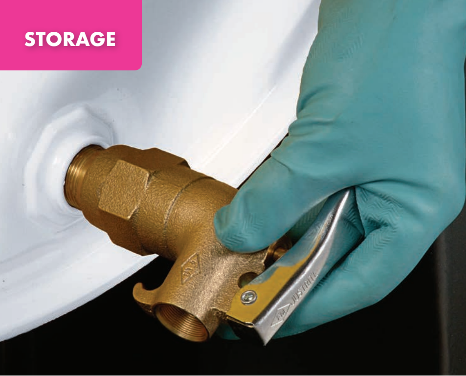
Above: Approved self-closing safety faucets incorporate an internal flame arrester which prevents flashback of fire into the drum.
