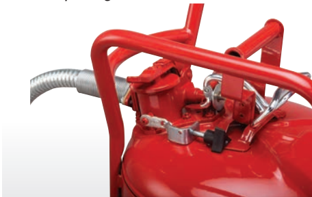
Type II D.O.T. Safety Can Two openings: top opening with lift lever for filling, and a second one with flexible metal hose attached for accurate, glug-free dispensing into smaller openings. Additional safety features include roll-bar construction and a fusible-link protected hold-down bracket for protection during over-the-road transport.
